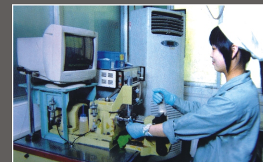
Computer-controlled spectrum analyzer for measuring bearing vibration
